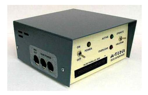
Power for the railroad tracks is derived from a 15 Volt AC 4 Amp transformer connected to the blue terminals on the rear panel of the DIU. The DCC output signal, used to both power and control locomotives on the layout tracks, is available at the green terminals, while a separate DCC output from the yellow terminals is taken to an isolated section of track for the purposes of programming the DCC decoders fitted in the locomotives -
