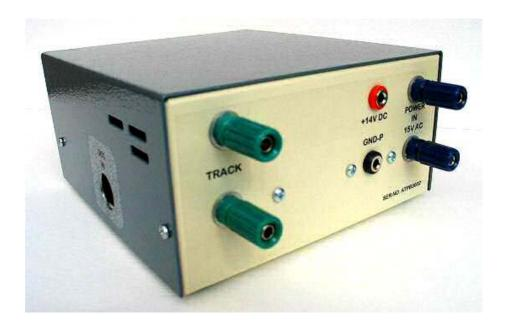
Internally, the circuitry of the PBU uses the same PCB as the DIU but the front digital section is omitted, and the rear output section is driven directly by a connection from the DIU or a preceding PBU. Several PBUs can be connected in series from a single DIU, which provides the necessary power for them all (see Section 11.3 of the User Guide for details) -
