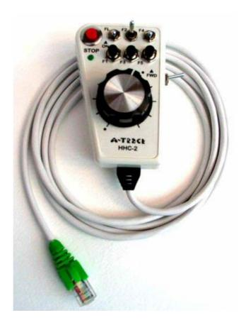
As explained in Section 11.2 of the User GUide, the A-TRACK HHCs are connected via their 8-way RJ45 jacks into a wired network driven by the Network Driver unit from the Atari 800XL Joystick Port 2. HHCs can be unplugged and then reconnected into any convenient point of the network as an operator moves around the layout - the locomotive assigned to that HHC continues to run under A-TRACK control at the last set speed while the HHC is disconnected.
