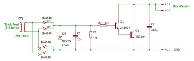
The small alternating input current, coupled from the DCC track feeder by current transformer CT1, is fed into a full-wave rectifier comprising diodes D1 – D4. The resultant direct current, smoothed by capacitor C1, then develops a voltage across resistor R1.
