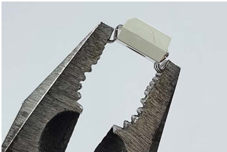
11. Adjust pin spacing of ODM1-4 chips gull-wing packages
