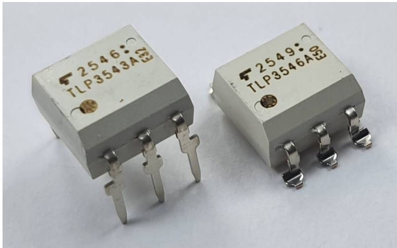
9. Dual-FET photorelay chip packages – dual-inline and gull-wing
